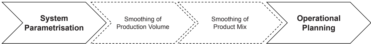
Fig. 2: Planning procedure of Heijunka-levelling
