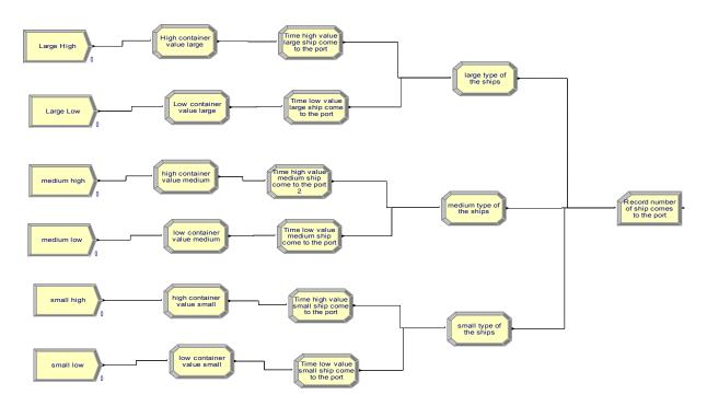
Fig 2:. Logic view of simulation model of berth process
