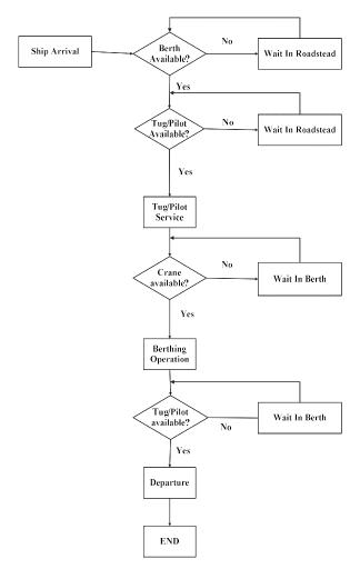
Fig 1: Ship berthing operation
