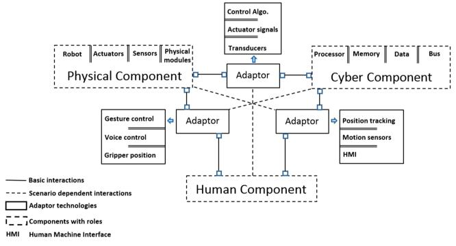
Fig. 1 Structure of CRCPS: detailed components, modules, adaptor technology modules and interconnected links
