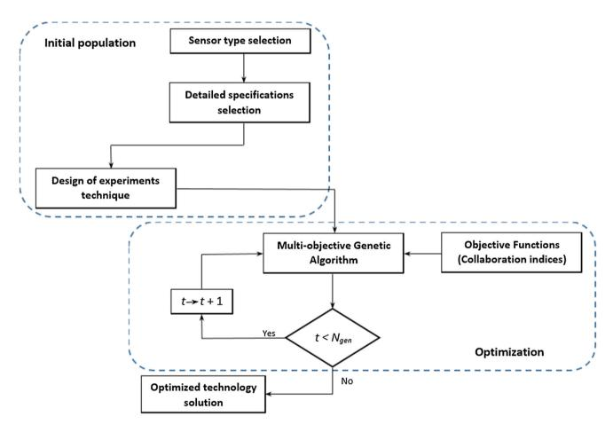
Fig. 6 Optimization data flow in CRCPS design methodology
